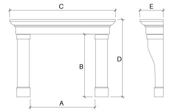
A: Opening Width - B: Opening Height - C: Overal Width - D: Overall Height - E: Depth
