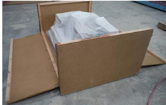
Figure 5: Remove plastic covering the pieces, and photograph the layout of the pieces for documentation.
