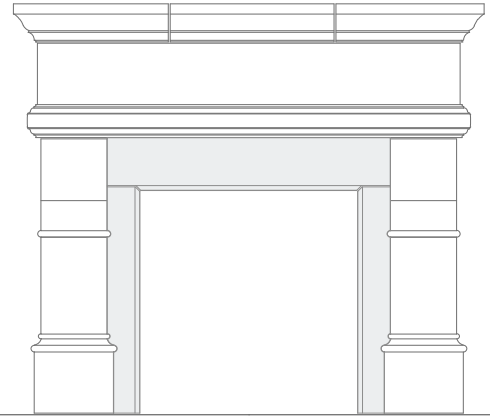
CHAMFER EDGE, STRAIGHT FILLER PANEL *
