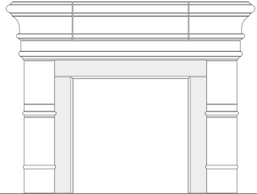
CHAMFER EDGE, STRAIGHT FILLER PANEL *
