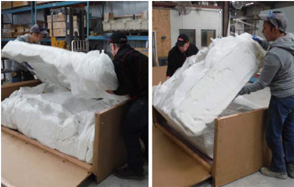
Figure 4: Lift monolithic foam straight up and over, there may be a top and sides or just one large piece.
