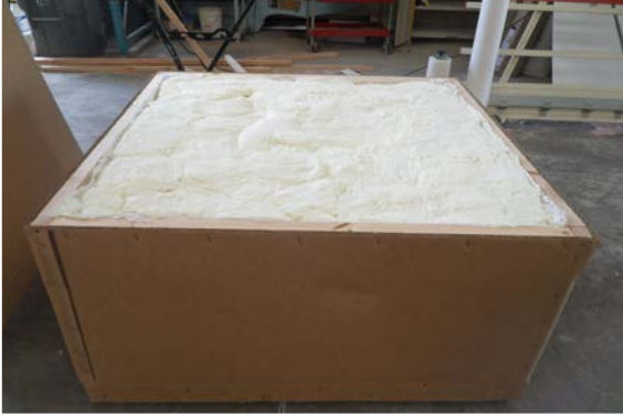
Figure 3. The crate is then shot with expanding foam to secure all parts as one in a monolithic package.
